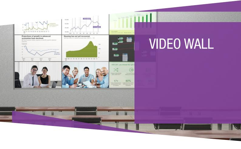
A video wall consists of multiple screens tiled together contiguously in order to form one large screen. Video walls can be easily found in control rooms, shopping malls, lobbies, etc. They allow distant passersby to view large images and nearby observers to read about small text.
